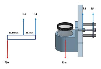
Both of these radial loads are far smaller than the load tolerance of bearing (57155k305), having 330lbs dynamic load capacity and 120lbs static load capacity.
