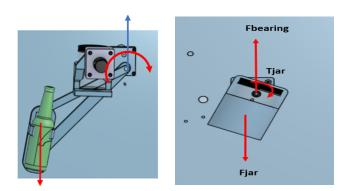
kg-cm. The torque is less than half of that of the bottle-motor system, allowing us to use a motor within a reasonable price range.
