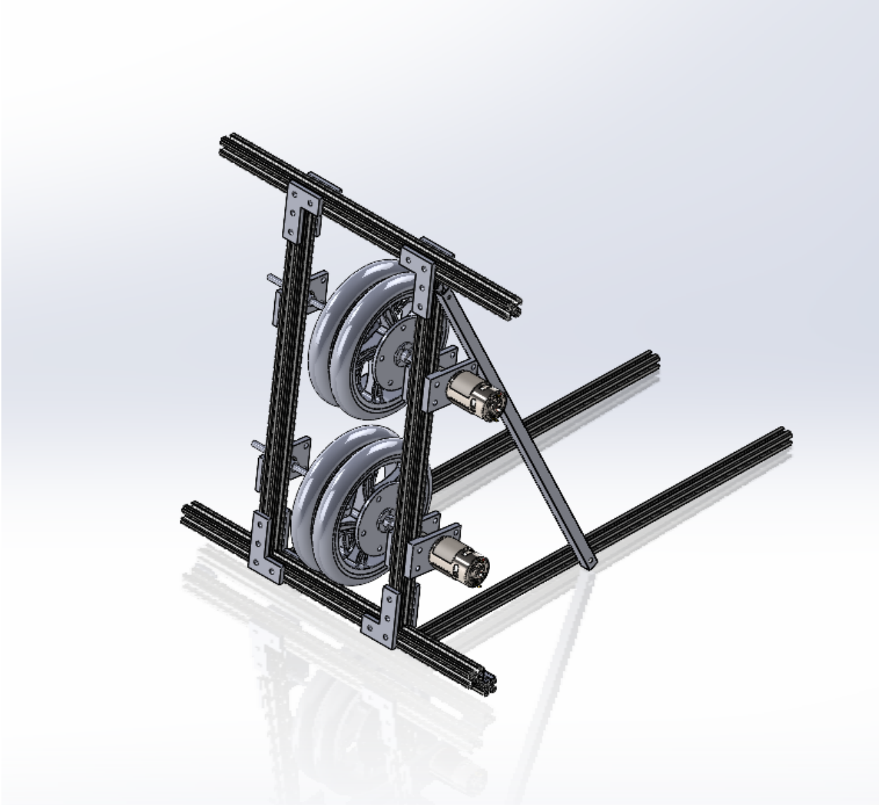
Figure 4: CAD of our shooter subsystem
