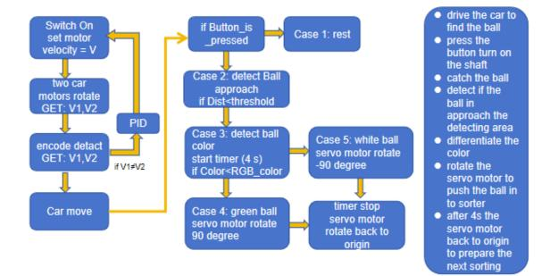
In the practical execution of the project, the set threshold for the color sensor had to undergo several tuning and adjustments. Initially, our goal was for the color sensor to detect any two selected colors. However, due to the physical constraints of the color sensor, it became necessary to establish distinct thresholds for the two balls, choosing colors from opposite spectrums—one light and one dark.
