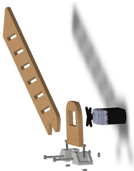
Figure 7: Exploded view of the sorting arms - dimetric view
