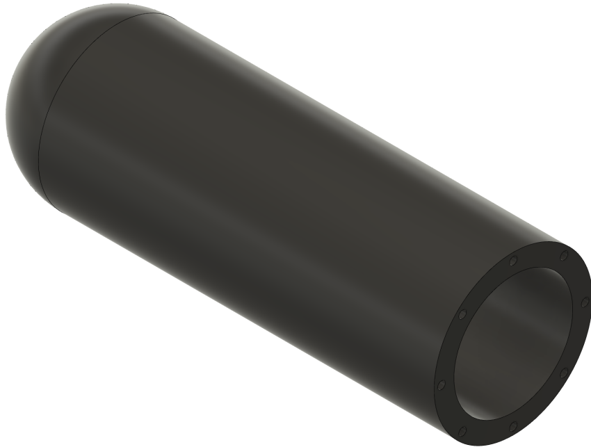
Figure 8: CAD - Isometric View of Delrin Hull (Watertight Compartment's Outer Shell).
