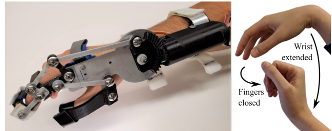
Fig. 1: (Left) The MWDO is worn the same way as a traditional WDO, but has an additional motor located at the proximal end of the device for adjusting hand behavior in parallel to the user's wrist motions. The fingertips are straight in the neutral pose in order to enable finer pinching motions. (Right) A tenodesis grasp demonstration shows how wrist extension closes the fingers, while wrist flexion allows the fingers to open.
