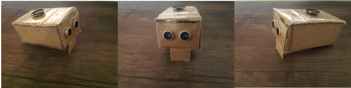
Figure 2: The device is shown from the left, front, and right sides. The ultra-sonic sensor and speaker can be seen protruding from the housing. The stand is deployed as to angle the sensor higher to detect the body of the dog rather than the paws.
