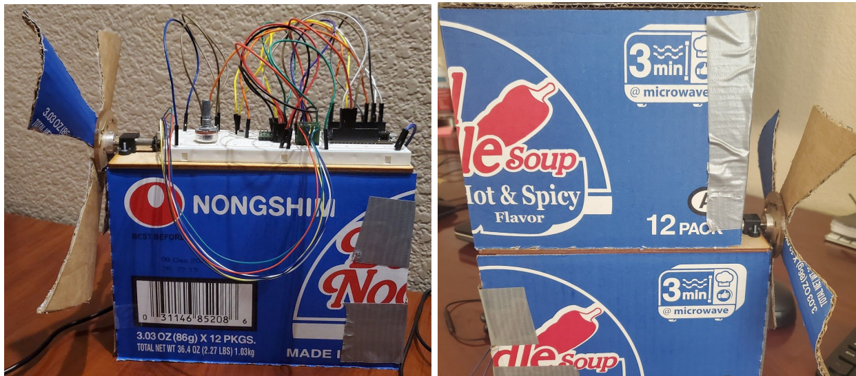
Figure 1: The cooling fan made out of cardboard is powered by a 5V power supply provided by a power cable that is plugged under the desk. On the left is the device without the housing and easier access to the breadboard for testing purposes. On the right is the device with the top housing for the circuit.
