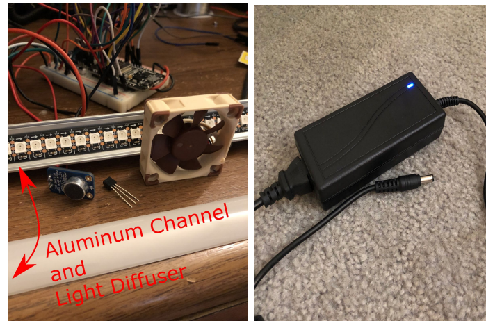
Figure 3. Circuit at a glance including the final mechanical component: an aluminum LED channel and light diffuser. Right image shows 40W power supplied used to power LEDs
