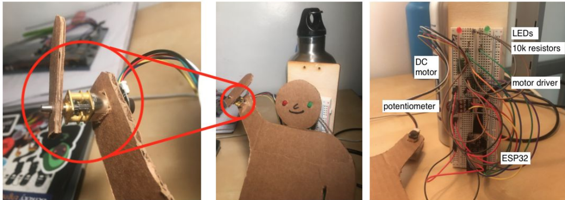
Figure 2: (Left and middle) Interface between the DC motor and cardboard figure. (Right) Circuit behind the cardboard figure, which is described in more detail in the following section.
