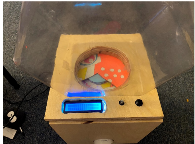
Figure 3: Interfaces for user include an LCD display, potentiometer, and pushbutton
