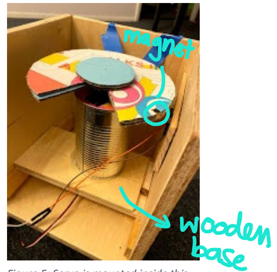
Figure 5: Servo is mounted inside this metal can which lies on a wooden base levitated by wooden spacers
