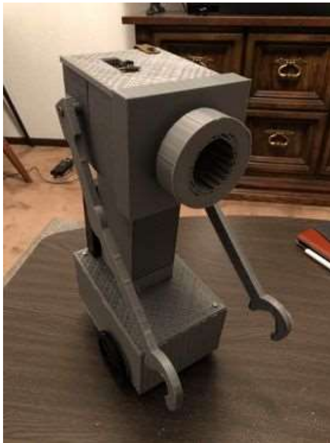
Figure 1: The Butter Buttlер automation device. The device is composed of a microcontroller, an infrared receiver module, two brushed DC motors, and a motor driver. All these components are secured within the 3D printed housing.
