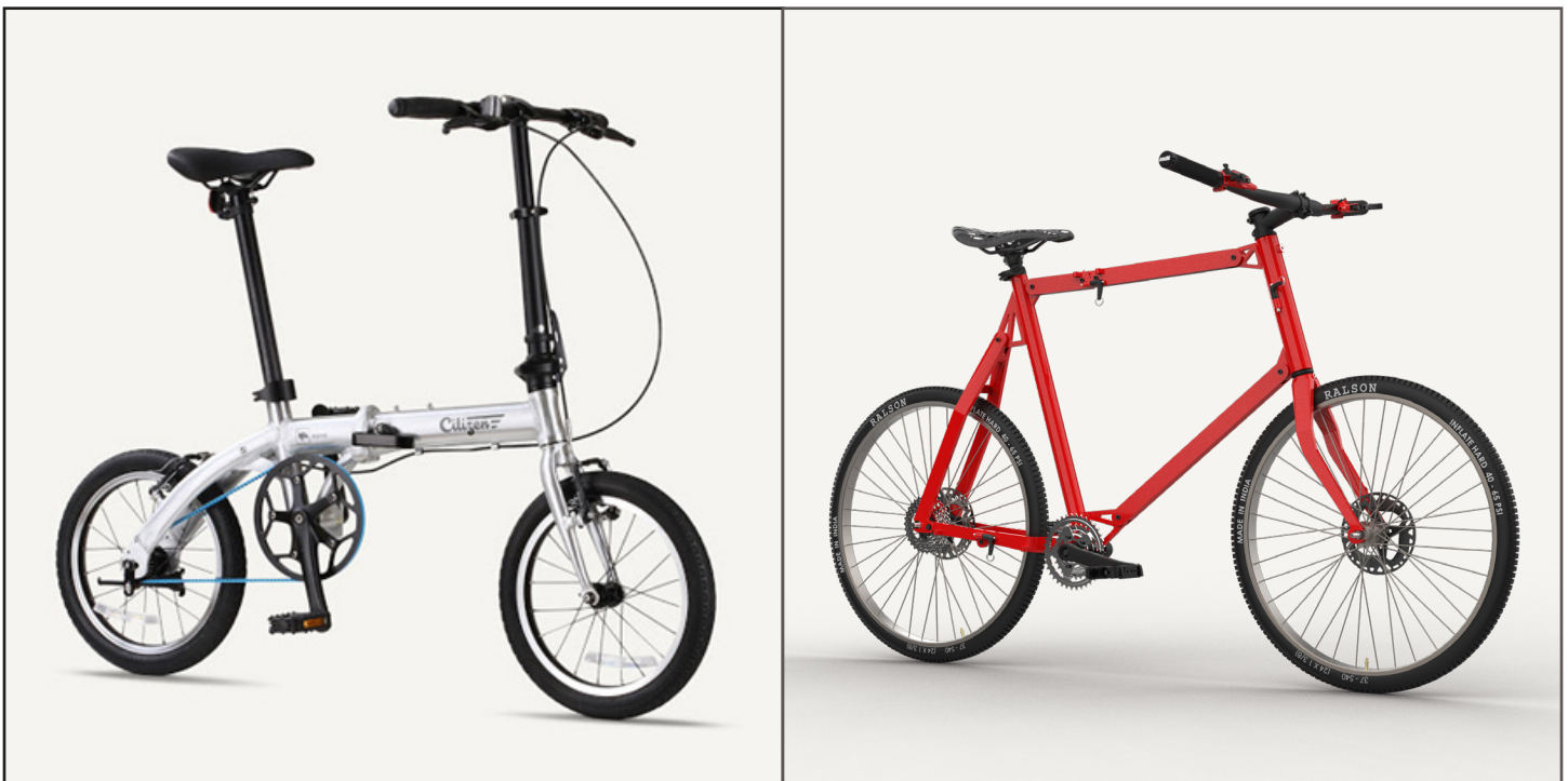
Figure 1: The ROME Citizen 16" bike (left) and the Edge Folding Bike (right). The new approach uses four and five bar linkages to collapse the frame into a thin bar.
