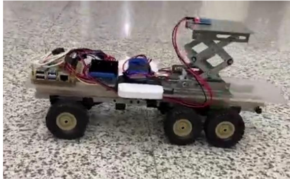
Figure 1: The cart with an air quality sensor on it(left). The elevator is attached to the cart, lifting the sensor up and down.
