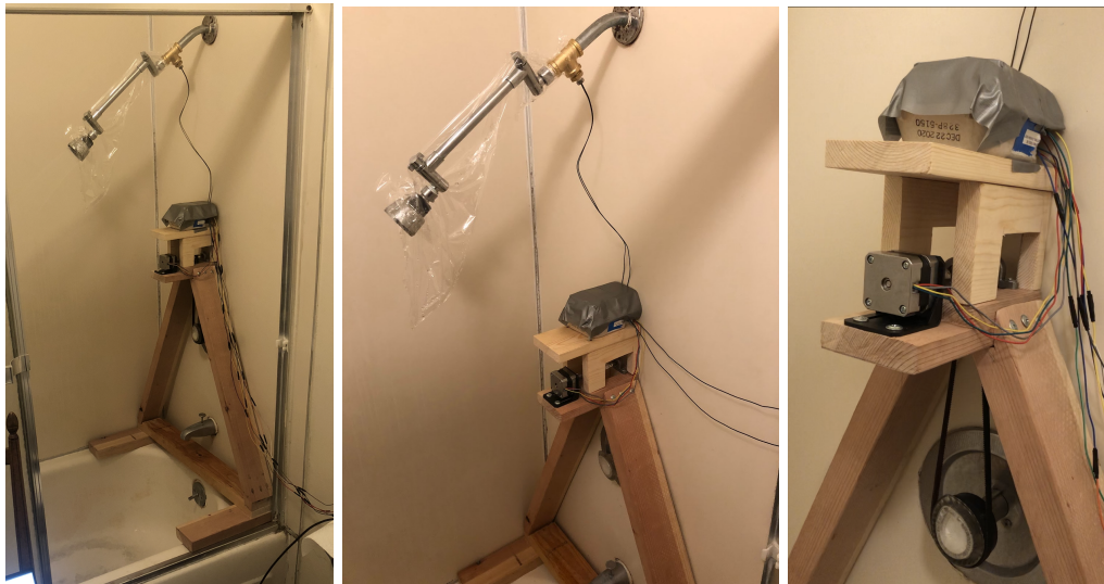
[Figure 1]: The shower temperature controller, note the high-tec seran-wrap and duct-tape-egg-carton drip guards to protect the breadboard and electronics.
