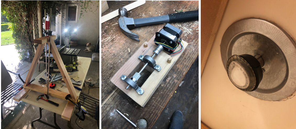
[Figure 2]: Going left to right, top to bottom, we have the wood frame mid-assembly, the motor and power transmission (note all the individual parts), the shower knob wrapped in sponge sealant, the timing belt around the timing pulley in line with the motor, and the front view of the stepper-knob power transmission.
