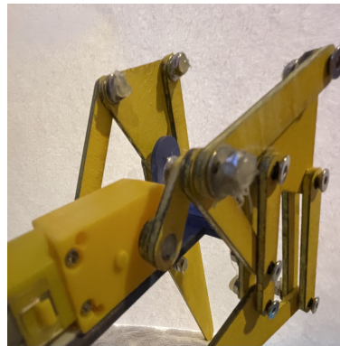
Figure 5: Side view of DC motor and Motor Connectors.
