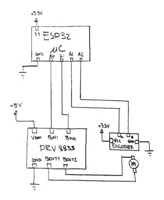
Aside from this final design, the circuitry went through several iterations that tested different mechanical and digital features. At first a MOSFET was used to run the motor and test if the mechanical side of the project could run and then a switch was used to rest the direction of rotation between ECU flashes. This was done to prevent damage to the motor as it would stall and short out if it tried to close already closed blinds or vice versa.
