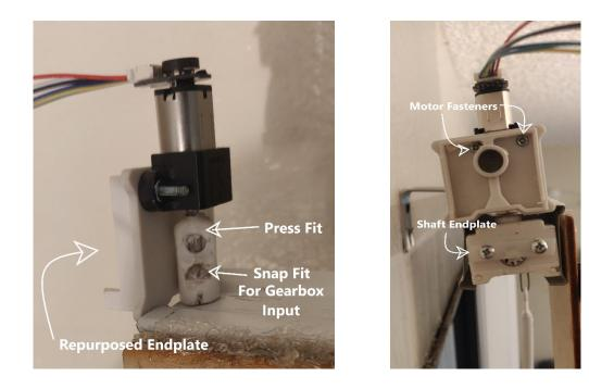
From the images, we can see an existing snap fit repurposed for double duty: holding the motor to the gearbox and keeping the gearbox from falling out of the hole in the frame rail. Additionally, since the end plate was repurposed as a motor mount, a new piece of plastic was used to prevent the splined shaft from working its way out of the side of the blinds.
