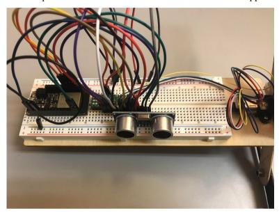
The distance sensor is used to send the activation signal to the arduino and its trigger threshold is set to 5cm. Then the arduino sends a motor signal to the encoder which controls the motor. This is a very simple motor control system just like what we learned in the lecture.
