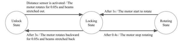
Showing above is the finite state diagram of the device.
