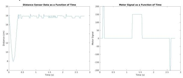
Showing above is the diagram of the data collected when the device is activated. From the distance sensor diagram, we could see when the distance sensor is activated. And from the motor signal diagram we could see how the encoder reacts to that which include a locking process, paper releasing process and a unlock process which represents the three signal changes in the diagram.
