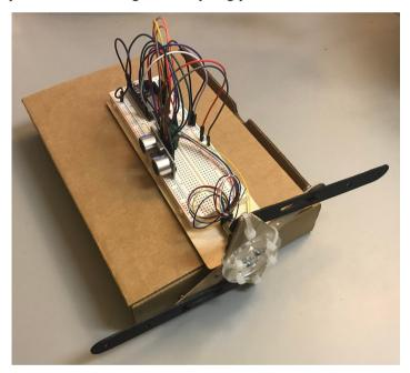
From the picture, we could see that this device is absolutely too big to fit into the toilet paper roll. And also, the distance sensor is facing the side which should direct along the axial to detect hands on the side of the roll. But that's the best I can get with the limited material I have at home. And hopefully, it clearly shows the idea of the project.
