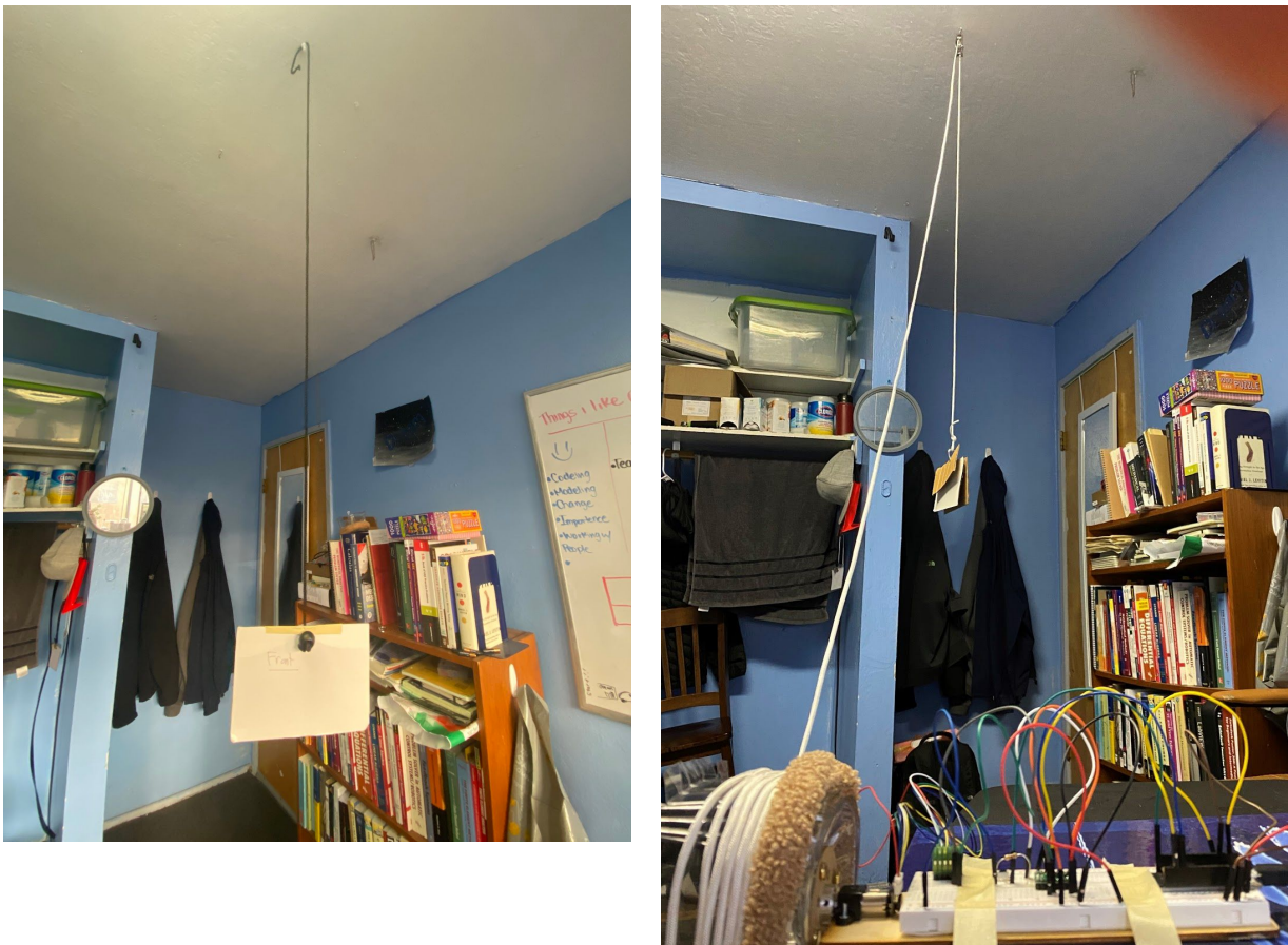
Figure 1. Left - before the automated system, this was the target used punching. Right- automated setup that moves the target up and down.
