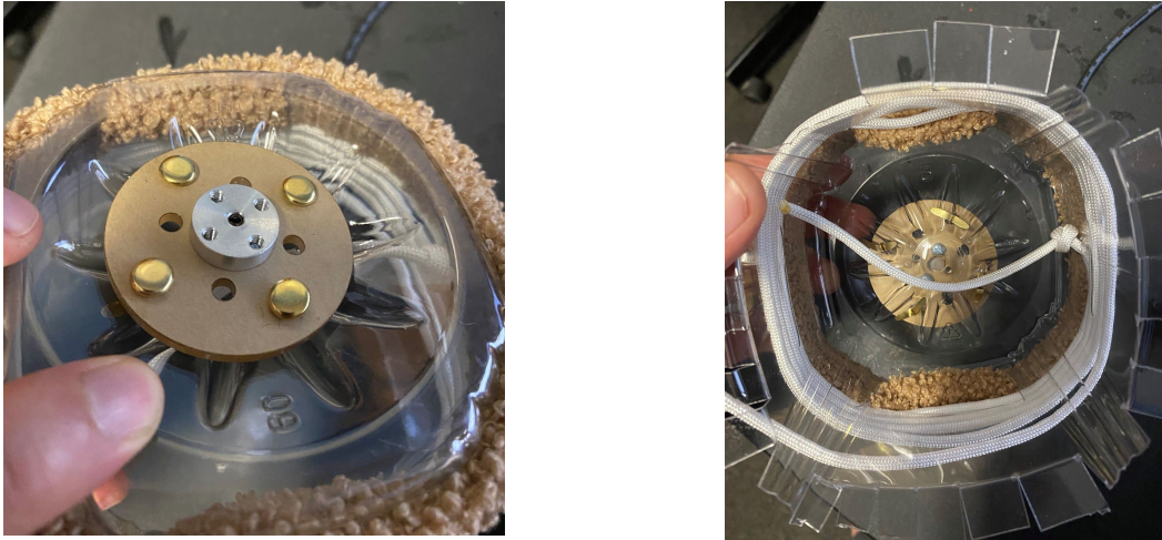
Figure 2. Plastic hub is attached to the aluminum hub by copper pins. The Aluminum hub is attached to the DC motor shaft
