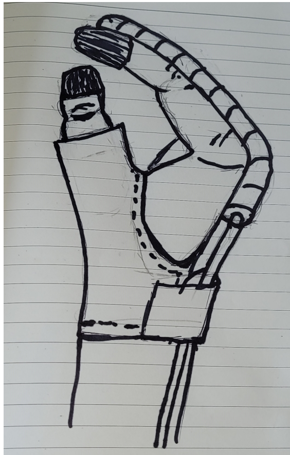
Fig. 7. Sketch of selected IMU controlled, soft robotic actuated, soft orthotic glove.
