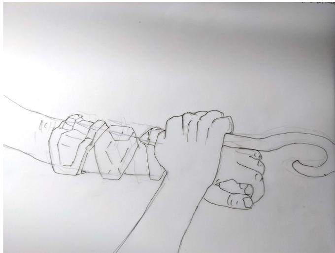
**c):**This demonstrates how to put on attachments (in this case a hook). The universal adapter has a mating port that the hook can fit in. The user simply needs to align the hook with the port to attach. The universal adapter will provide 1 degree of freedom(rotation)
