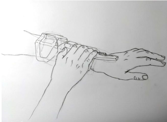
**e):**When the user wants to detach the attachment, simply press the button on the middle of the universal adapter. The adapter will release the attachment automatically.
