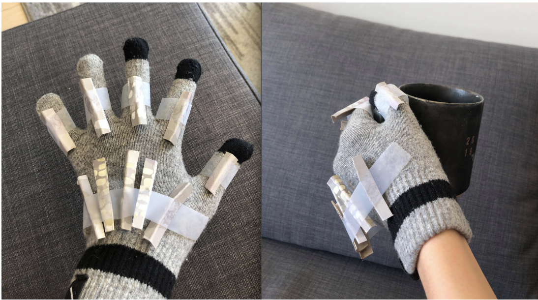
Fig. 5. Non-functional prototype showing exoskeleton structure (left) and use holding a cup (right)
