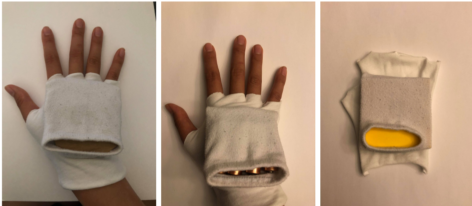
Fig. 6. Testing the heat pack size/shape so that it does not interfere with dexterity.
