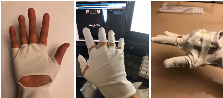
Fig. 7. Testing for need of palm tactile sensitivity and potential attachments to fingerless glove.
