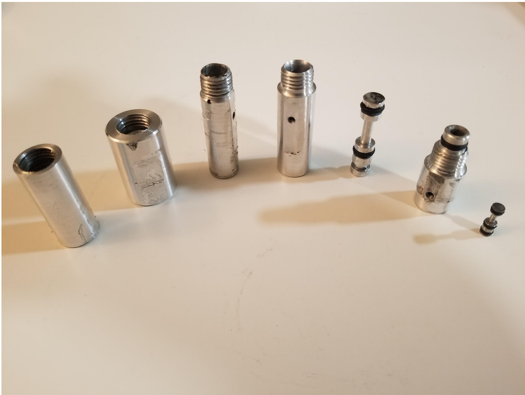
Pyro valve body prototypes and final design
