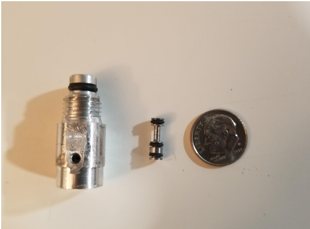
Valve body and plunger with a dime for scale
