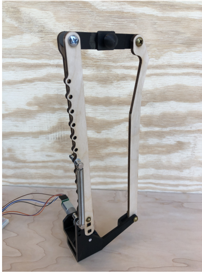
Fig. 4: Stabilizing arms functioning in the full assembly.
