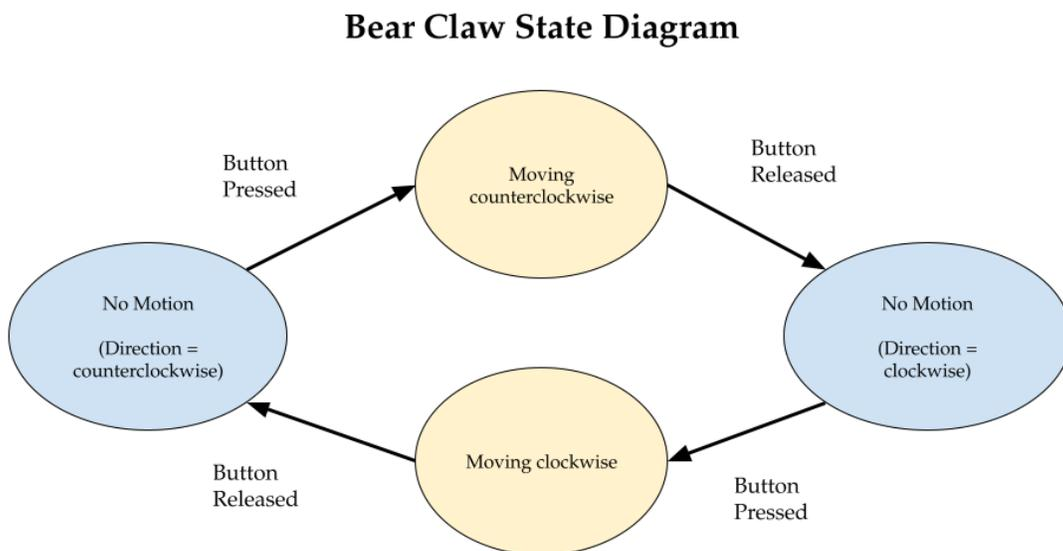
**Fig. 1:** State transition diagram for operation of the externally powered design (motorized claw).
