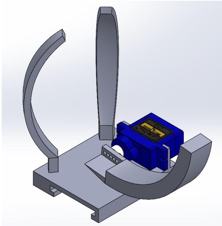
**Fig. 6:** Full Bear Claw mechanism with the motor, final claw, and static claws.
