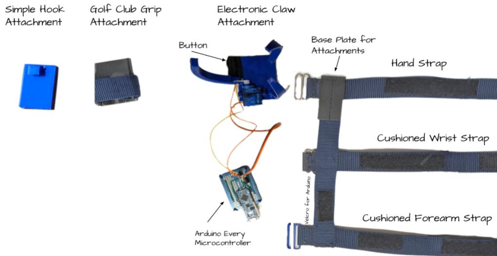
**Fig. 7:** Full device showing the hand straps and the three different attachments (hook, golf club grip, and motorized claw).
