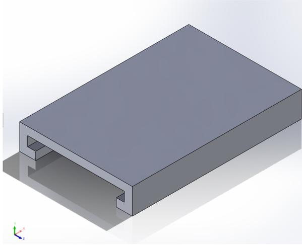
**Fig. 3:** *Blank attachment that is slid over the base*
