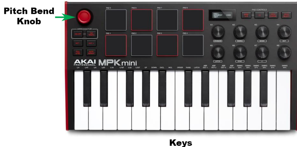
Fig. 1. The MPKMini MIDI piano keyboard, owned by the need-knower, is a good example of a normative MIDI piano keyboard. [2]
