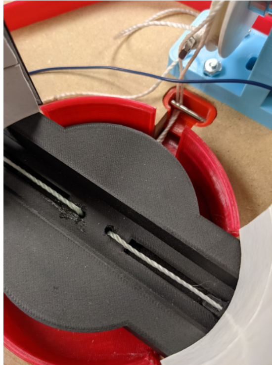
Fig. 6: The holes for the string to route through the gripper frame may be increasing the friction of the system.
