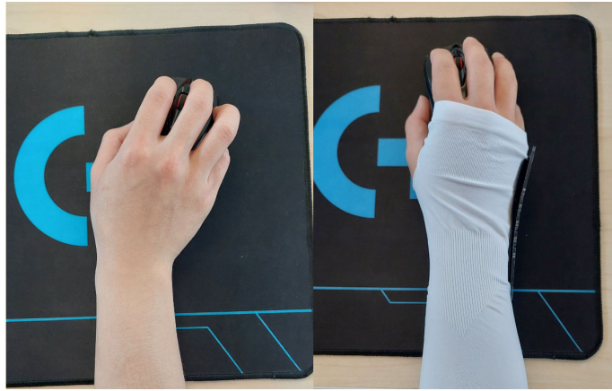
Fig. 6. Without the sleeve, the user’s wrist naturally deviated to the ulnar section in the rest position. With the sleeve, the user’s hand became straightened with the arm
