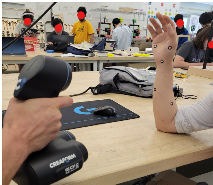
Fig. 9. Scanning the shape of the forearm to create the shape for the wrist support.
