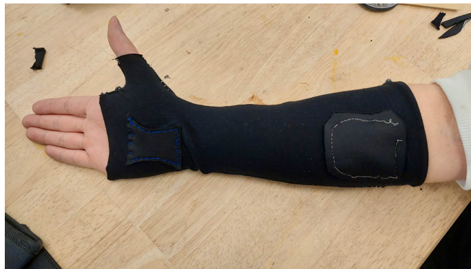
Fig. 7. This first generation arm sleeve prototype provides support for the palm and a smooth surface beneath the arm.
