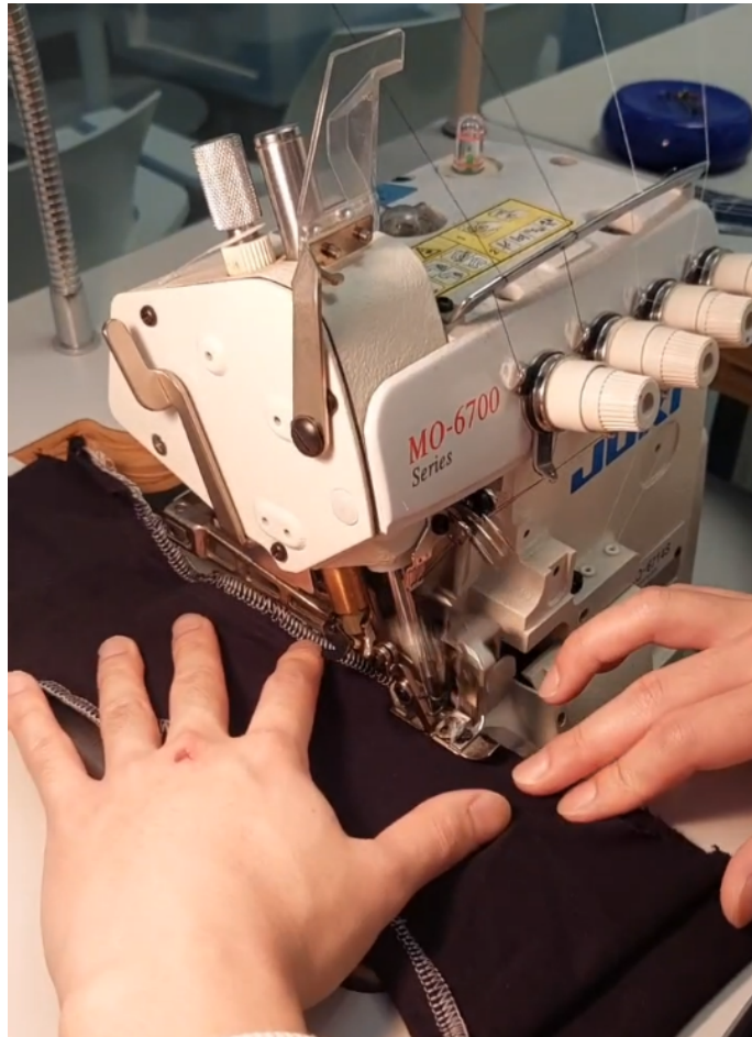
Fig. 8. Sewing together the lycra fabric to be form fitting, comfortable and ready for mounting our hardware.
