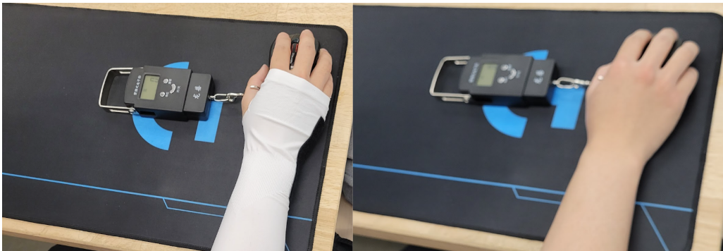
Fig. 3. Friction test setup. The left shows the test with the sleeve on, whereas the right shows the test without the sleeve.
