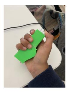
The casing design was manufactured through 3D printing in two separate parts. The curve was added onto the external part of the design to ensure a better grip on the pencil, which is an intentional contrast to the single tip stylus and slate, which is skinny in frame and harder to grip. The design also caves inwards from sides of the pen, for those who choose a traditional grip.
