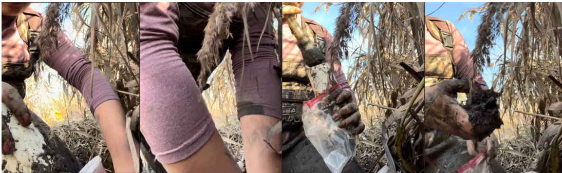
Fig. 2. Progression of how to collect a mud sample. A custom PVC pipe tool is inserted into the ground, the researcher pushes tool into the ground, the sample is removed with additional tool, and additional sample is added to the collection bag.
