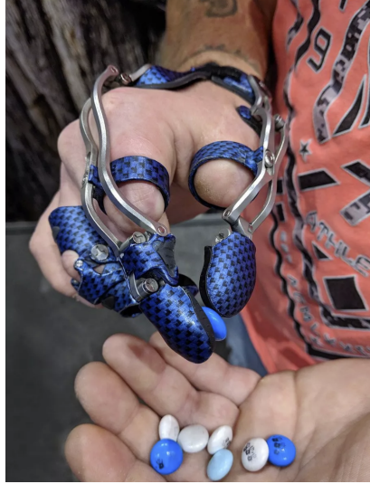
Fig. 1. Naked Prosthetics, ThumbDriver product that is used to help finger amputees regain function of the distal phalanx of the thumb with use of the thumb's proximal phalanx as the actuating input [6].
