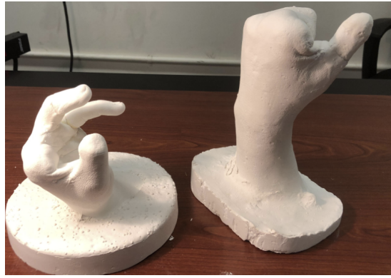
Fig. 4. Hand castings of interviewee, on left it shows the left hand casting in an open configuration, and on the right the left hand casting is in a fist shape with thumb sticking out. The casting on the left will be used for testing fitment of the index and middle fingers, while the casting on the right will be for fitment of the distal phalanx for the thumb.
