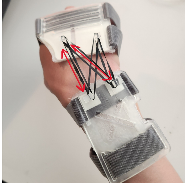
Fig. 6: Prototype spring damping diagram
