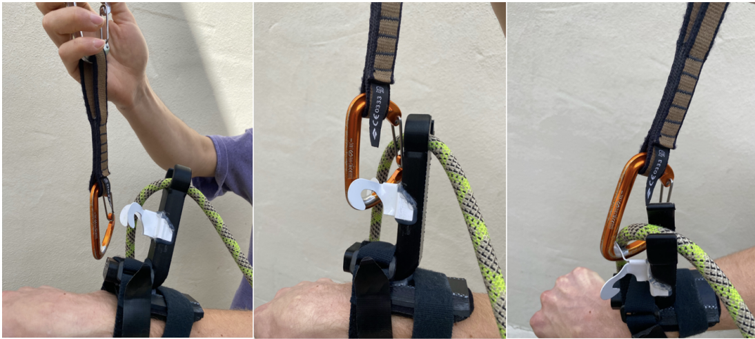
Fig. 3. A progression of clipping with the proposed device. The bottom hook will stabilize the carabiner and the rope will rest in the rope notch.
