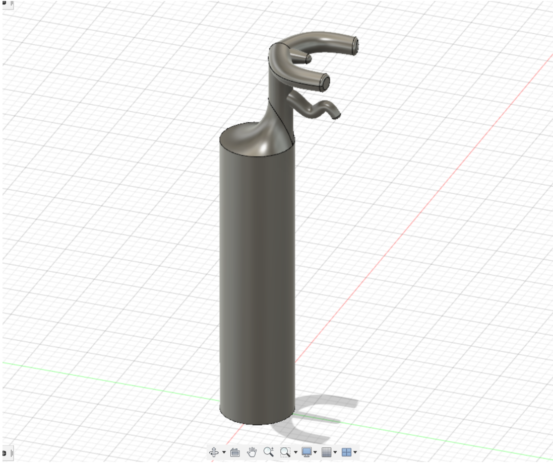
Fig. 4. This is our initial prototype design. It is made to be held with a hand to test the clipping mechanism, which would later be arm-mounted.
