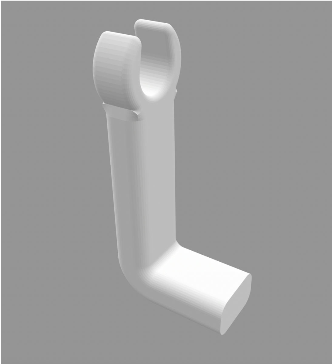
Fig. 5. This is our prototype design once we tested the optimal geometry of the clip. It is the rope notch that holds the rope. The metal hooks and arm-mount are attached at the neck and base, respectively.
