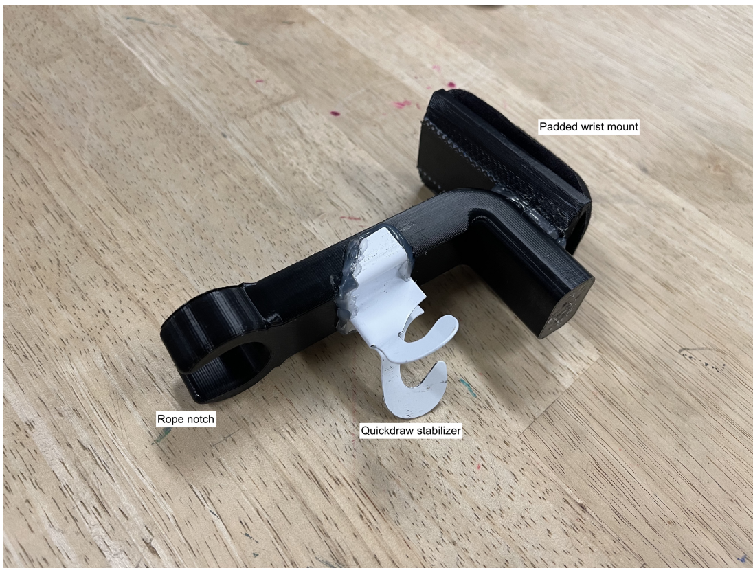
Fig. 1. Our first functional prototype. The white hook is placed in the quickdraw and the rope nests into the black notch.
