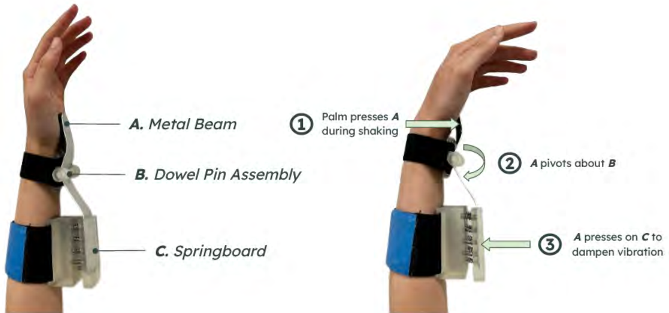
Fig. 2: The proposed devices features a spring board connected to an angled metal bar, creating a seesaw mechanism that absorbs vibrations in the flexion/extension direction of the wrist.
