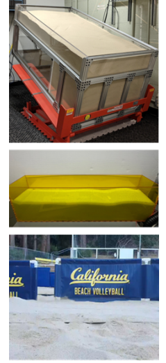
(b) Granular Media Testbeds (top to bottom): MARS90, Glass Beads, and Beach Volleyball Court.
